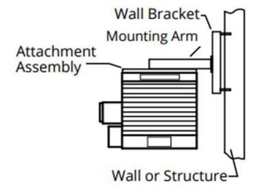
HLWM Wall Mounting Kit Ideal for use in buildings that have substantial walls. Arm only can also be bolted directly to structural steel.
