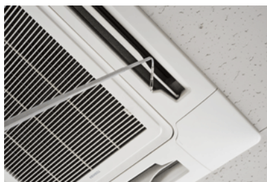
Telescopic articulating probe makes measurements in hard to reach places
