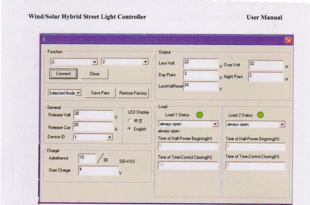
(Street Light Controller Parameters Setting Interface)
